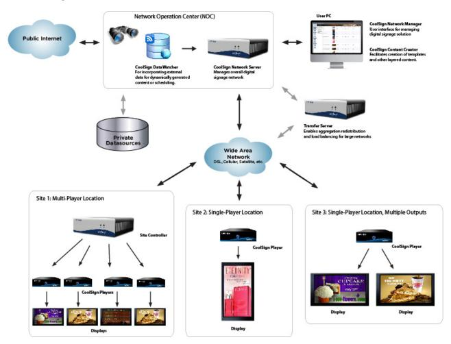
**CoolSign Network Server:** The core of any CoolSign network - available in various capacities to fit the needs of networks from small to large; the main repository for all network data and controls the actions of all other devices on the network. There is always one and only one CoolSign Server per network.
